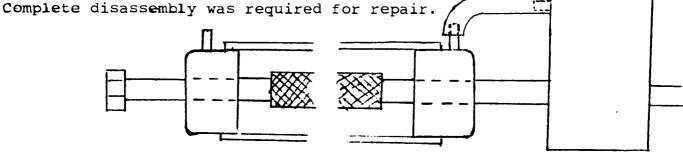
"Luckily, I found an extremely knowledgable welder who diagnosed the cracking and deterioration as electrolytic corrosion. He was able to normalize the flange with an acetylene torch and restore it to "as new" condition.
