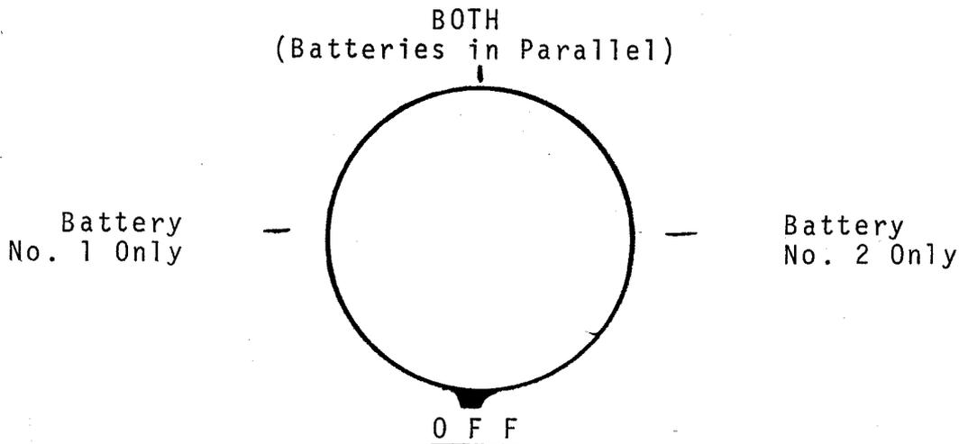
Battery charging is dependant upon your selection by means of this switch (i.e. to the left Battery 1 only, to the right Battery 2 only or up both batteries in parallel), when the engine is running. The (Opt.) converter charges independent of this switch.
