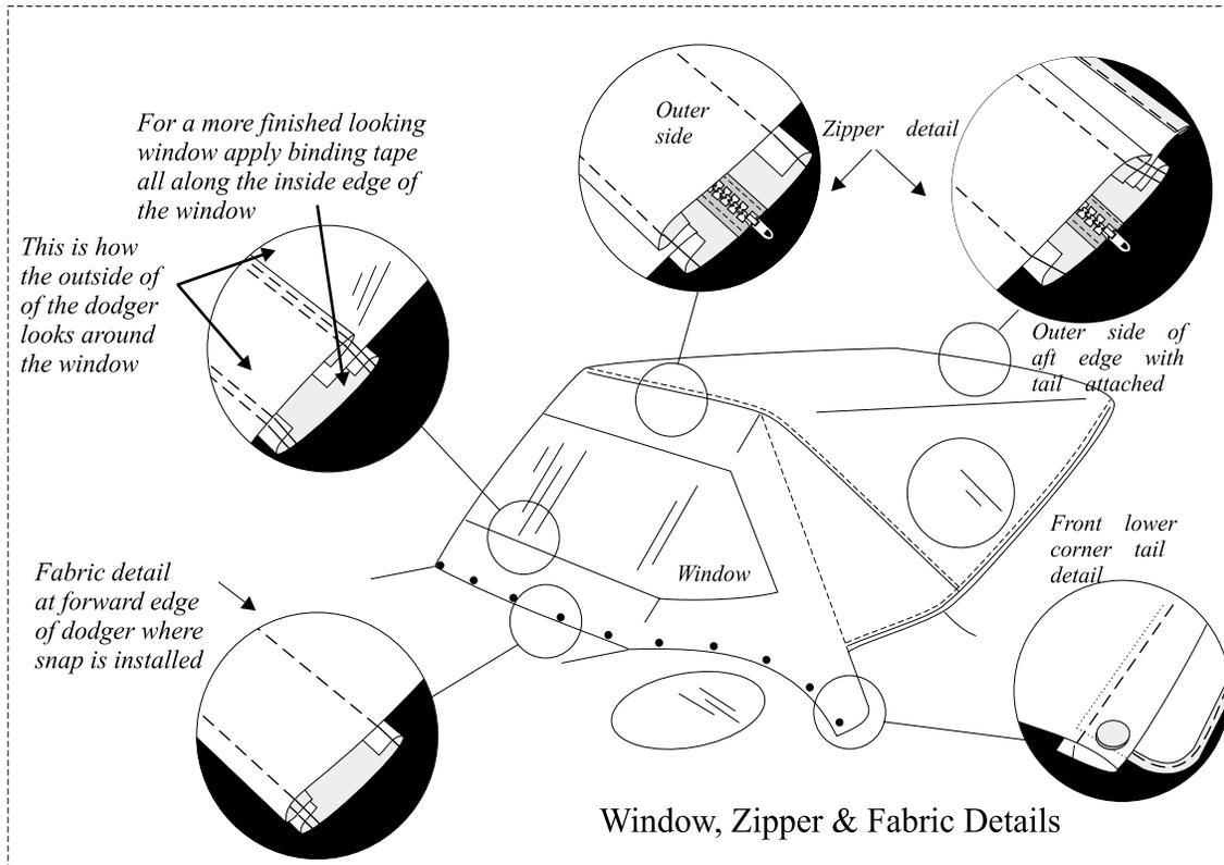
cover fabric. Run a row of stitches (straight or zigzag) all round the window. Keep the vinyl down while sewing—otherwise it will tend to break free and form a bubble in front of the presser foot because it is so sticky. (If you have a walking foot machine, the plastic can be up when you sew.)
