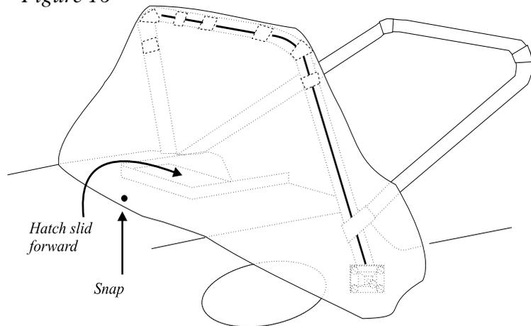
*If the hatch slides under the boat's deck, mount snaps right in front of the hatch cover.*
