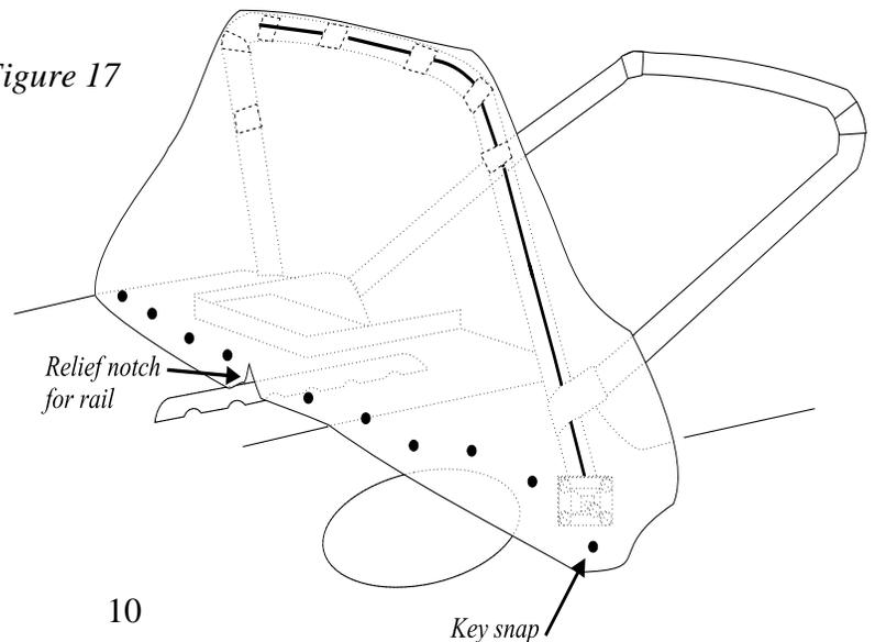
rails and any other protrusions on the cabin top (Figure 17). The last snap should be located on a line extended from the longest bow leg (Figure 18). Any snap mounted aft of this location would have to be undone in order to fold the frame forward.
