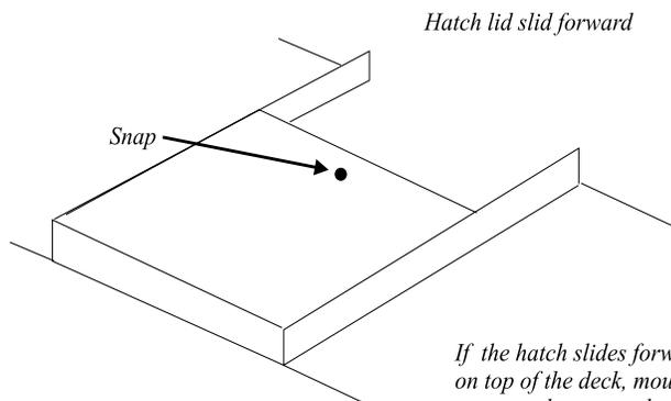
*If the hatch slides forward on top of the deck, mount the snaps to the outer edge of the hatch.*
