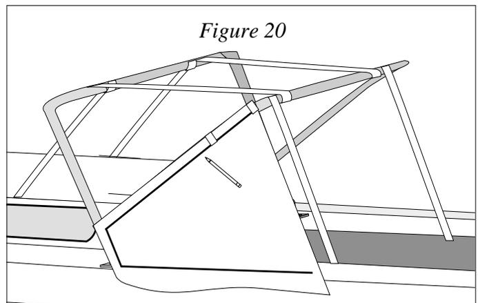
Tape curtain blank in place and mark with marking pen
