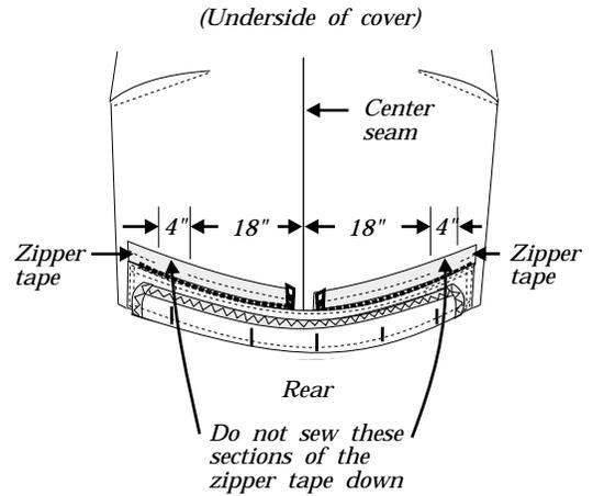
Sew a 7/8-inch wide binding tape all round the Bimini. This will finish all the exposed edges. We like to use a zigzag stitch for this binding, but a straight stitch can also be used if you are careful to place it near the inside edge of the binding on a consistent basis.
