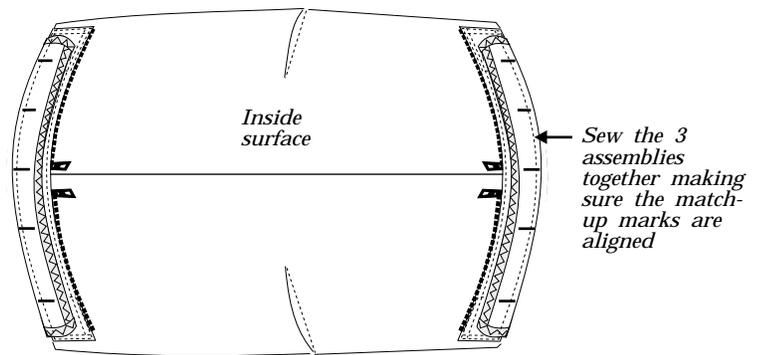
Sew the 3 assemblies together making sure the match-up marks are aligned
