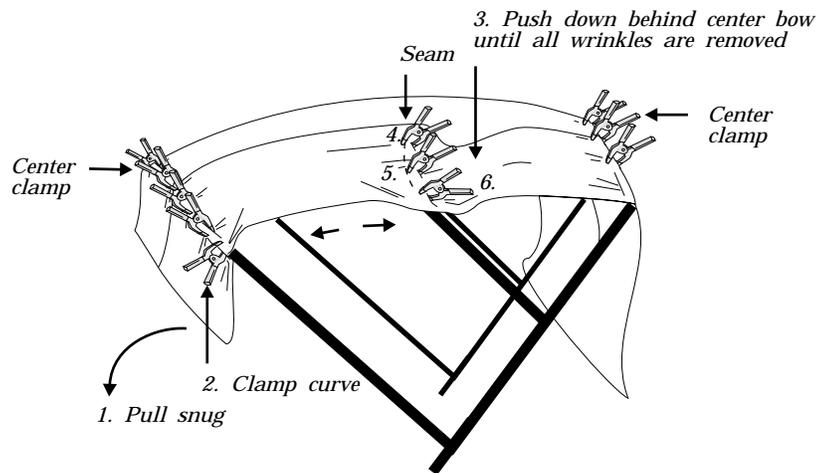
*Clamps 4, 5 & 6 - Clamp the cloth then pull cloth towards the curve of the center bow. Continue this process after each clamp insertion.*
