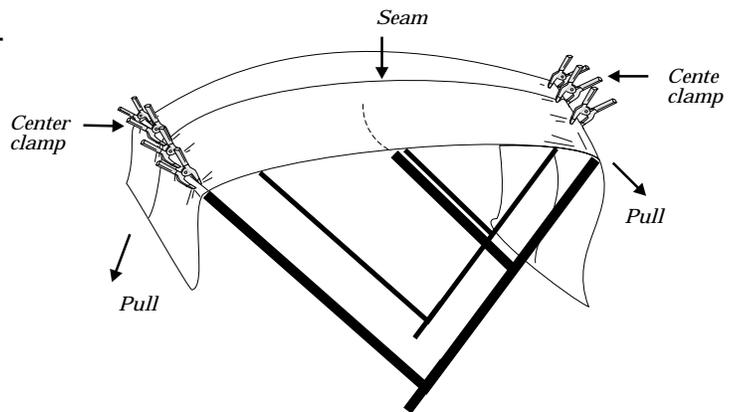
Start at the centered clamps and stretch the cloth out between the forward and aft bows. Clamp along the bows on three to six-inch intervals drawing the fabric tightly as you go.
