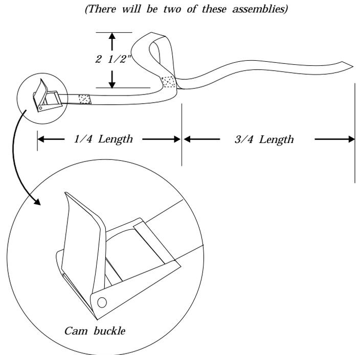
The fore and aft straps should be cut 3 times the length from the mounting point of the frame up the leg to the edge of the cover. Sew
