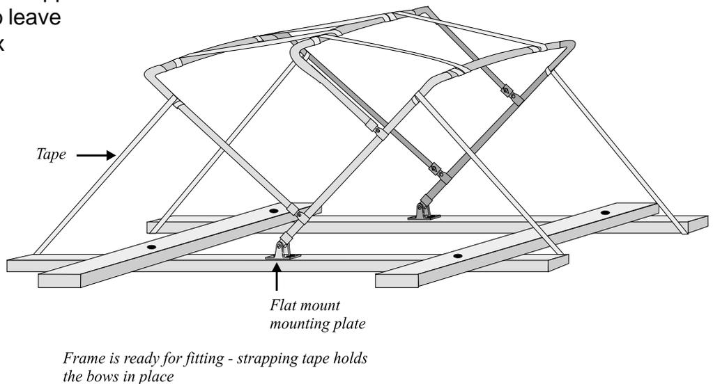
After cutting the frame width, tape the bow assembly back together. Be sure the spline tubing is inserted equally in the leg and the center piece and that the center piece (if crowned) is up.
